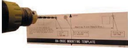
2. Drill two mounting holes ( $\varnothing$  3.4mm or 1/8").
